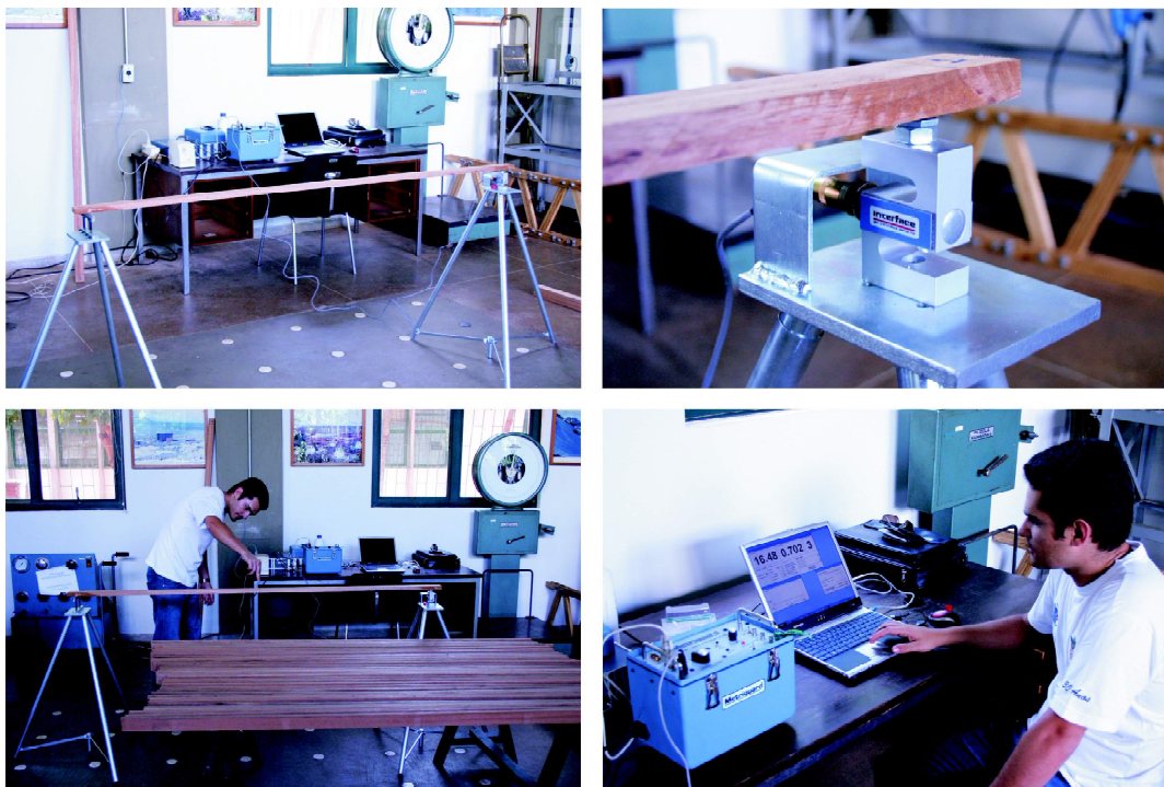
Figure 1 – Nondestructive testing by transverse vibration.
