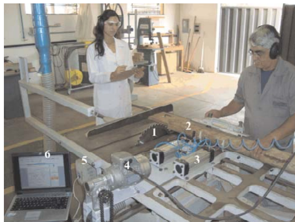
Figure 1 – Feed rate and cutting speed controlled moving circular saw (DCF/UFLA). 1) circular saw, 2) log section, 3) pneumatic pistons, 4) feed motor, 5) variable frequency drive and 6) computer.
