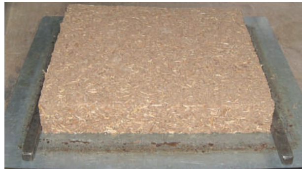
FIGURE 1 Photograph of fiberboard mat formation, ready to be put under the hot-press.
