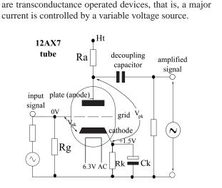
Figure 2: Common cathode circuit.
