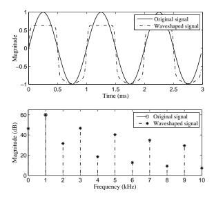
Figure 9: A 1 kHz sine wave filtered by Eq. 3 in the time and frequency domains.
