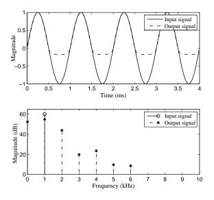
Figure 13: A 1 kHz sine wave filtered by Eq. 5 in the time and frequency domains.
