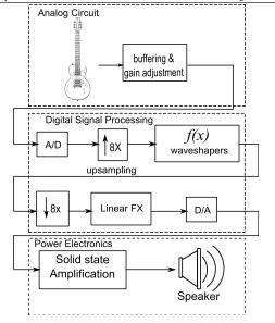
Figure 12: Block diagram of a DSP system for simulating vacuumtube amplifiers [10].
