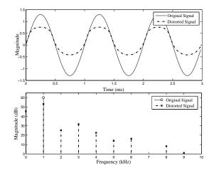
Figure 11: A 1 kHz sine wave filtered by Eq. 4 in the time and frequency domains with parameters a = 0.3 and b = 0.7.
