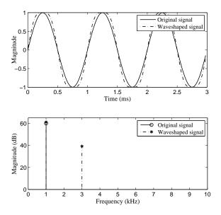
Figure 6: A 1 kHz sine wave filtered by Eq. 1 in the time and frequency domains.
