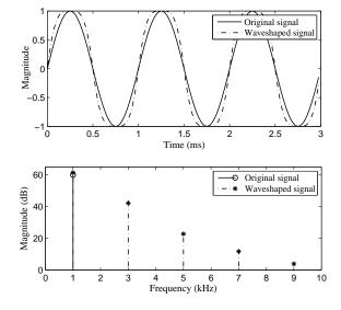
Figure 8: A 1 kHz sine wave filtered by Eq. 2 in the time and frequency domains.
