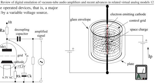
Figure 3: Electron flow inside tube.
