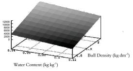
**Figure 2.** Surface response for penetration resistance (*PR*) related to the density (*D*) and water content (*WC*) of the soil.
