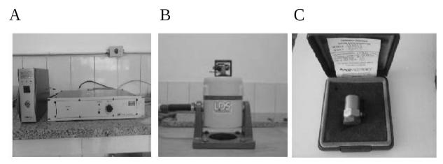
**Figure 2.** System used in vibration trials: (A) signal generator COMET<sub>USB</sub> and PA100-CE amplifier, (B) electromagnetic shaker and (C) piezoelectric acceleration transducer employed on system control.
