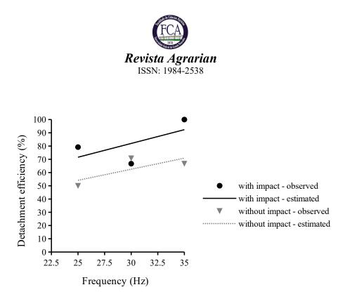
**Figure 9.** Effect of the mechanical vibrations trasmission, with or without impact, over the detachment efficiency of the coffee fruits.
