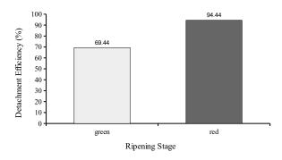
**Figure 6.** Effect of the ripening stage over the detachment efficiency of the coffee fruits obtained from the Trial 2 (mechanical vibrations transmitted to the coffee fruit-stem system due the impact of a rigid rod).
