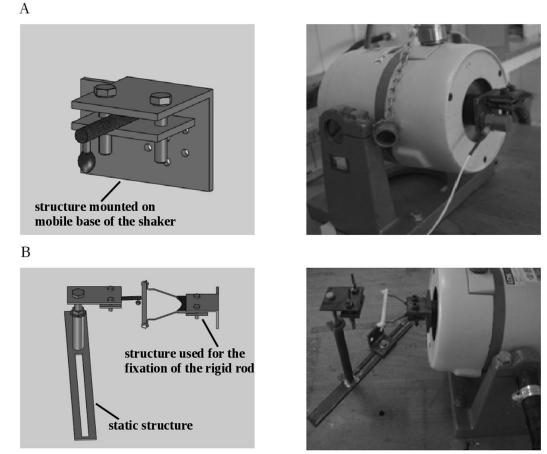
Figure 3. Representation of the two configurations of the vibration trials and its respectively fixation structures: (A) structure mounted on the mobile base of the shaker used on vibration trials without impact and (B) static structure for samples fixation and structure used for fixation of the rigid rod used on vibration trials performed by using impact over the coffee fruits.
