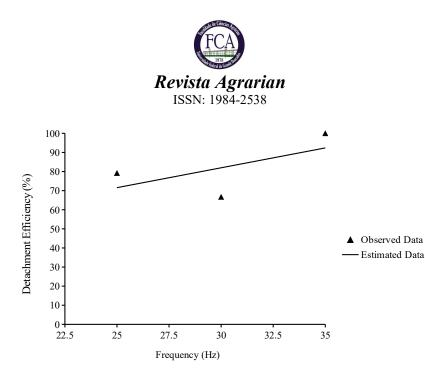
**Figure 5.** Effect of the frequency of vibration over the detachment efficiency of the coffee fruits obtained from the Trial 2 (mechanical vibrations transmitted to the coffee fruit-stem system due the impact of a rigid rod).
