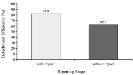
**Figure 8.** Effect of the mechanical vibrations transmission over the detachment efficiency of the coffee fruits obtained from the Trial 3 (mechanical vibrations transmitted with or without impact of a rigid rod on the coffee fruit-stem system).
