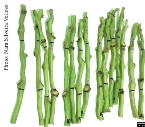
Figure 1. Samples of rachillas cut from macaw palm bunches and used in the traction tests.
