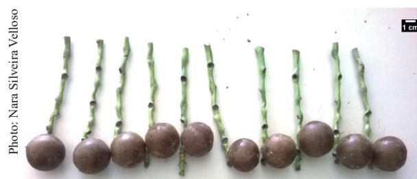
Figure 2. Samples of rachillas with one fruit cut directly from macaw palm bunches and used in vibration tests.
