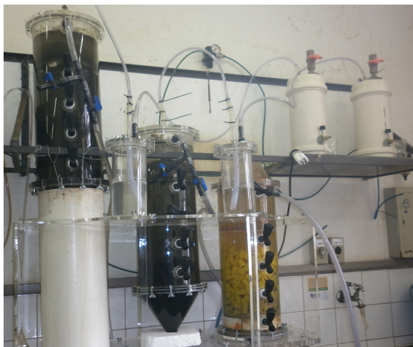
Figure 1: Treatment system on a laboratory scale – UASB reactors in series with one ASBF.
