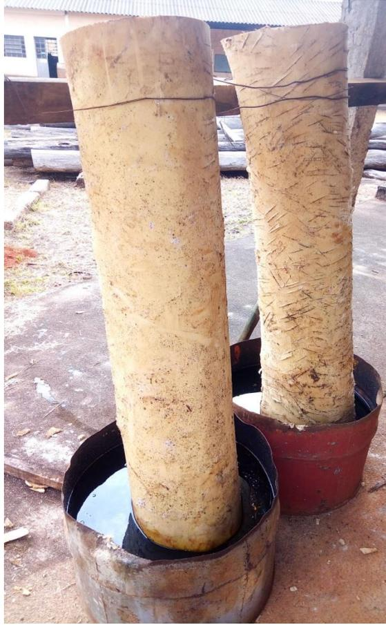
**Fig. 1.** Treatment of the logs with CCB by the sap-displacement method.
