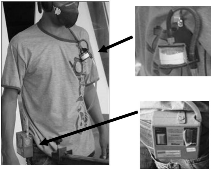
Figure 3. Placement of the individual collection of airborne dust showing details of the cassette with PVC membrane filter and the gravimetric pump position on the worker. Source: Field research.
