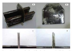
**Figure 5.** Apparatus developed for the shear test (A), blade used for test (B), without tensioner (C), and blade with tensioner and 45° chamfer at the end (D).
