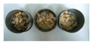
**Figure 1.** Crucibles containing chopped samples of macaw palm rachis with a volume of 1 cm<sup>3</sup>.
