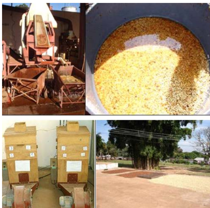
Fig. 1 Processing and drying of natural coffee in mechanical dryer and yard.
