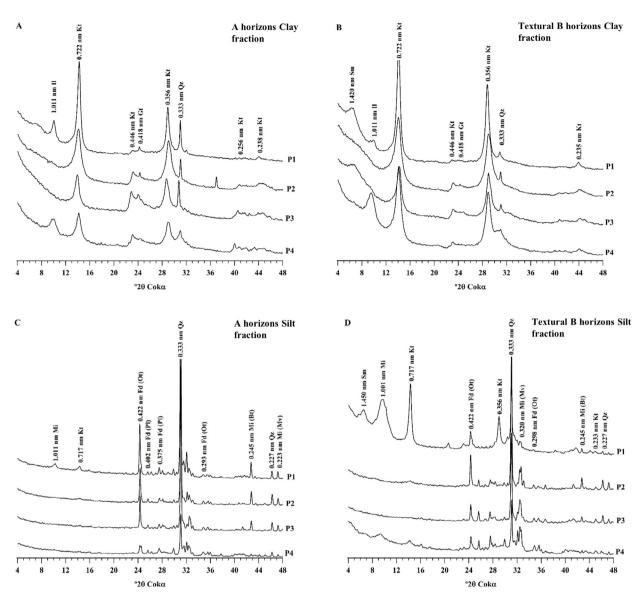
**Figure 2:** X-ray diffractograms of the Luvisols. A: Clay fraction of A horizons. B. Clay fraction of textural B horizons. C. Silt fraction of A horizons. D. Silt fraction of textural B horizons. Sm - smectite, Kt – kaolinite, II – illite, Hb – hornblende, Mi - mica, Bt - biotite, Mv - muscovite, Fd - feldspar, Ot - orthoclase, PI - plagioclase, Qz – quartz.
