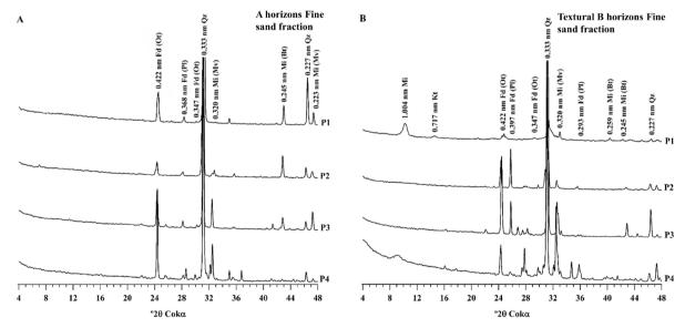
**Figure 3:** X-ray diffractograms of the fine sand fraction of the Luvisols. A: Sand fraction of the A horizons. B. Sand fraction of the textural B horizons. Kt – kaolinite, II – illite, Hb – hornblende, Mi - mica, Bt - biotite, Mv - muscovite, Fp - feldspar, Ot - orthoclase, PI - plagioclase, Qz – quartz.
