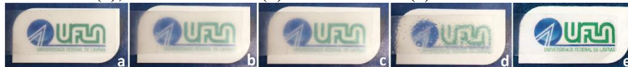
Figure 10 - Visual aspect of WPI film (a), 90W/10P blend (b), 80W/20P blend (c), 70W/30P blend (d) and PVA film (e).
