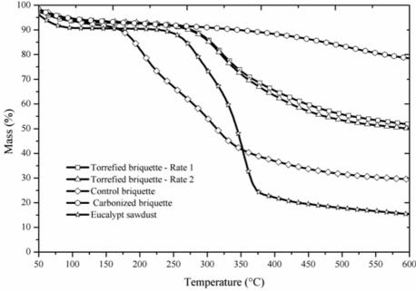
Figure 1 – Mass loss in function of temperature of the analyzed fuels.
