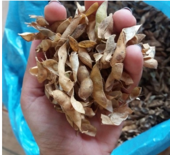
Figure 1. Soybean pod husks used in the production of medium density particleboards.
