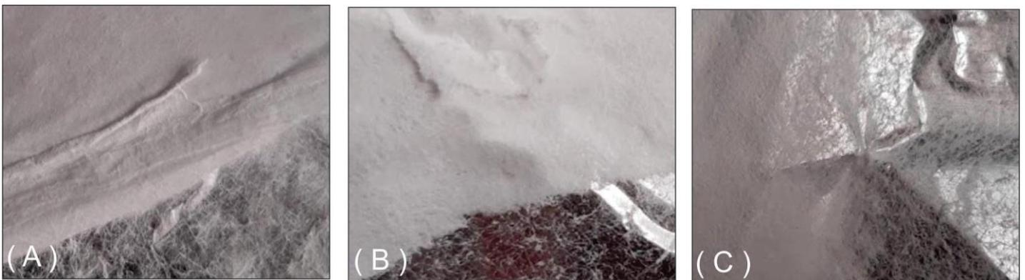
**Figure 2:** Nanofibrous mats of (A) PBAT/PVP-0, (B) PBAT/PVP-25, (C) PBAT/PVP-50. The PBAT/PVP-75 and PBAT/PVP-100 samples did not form nanofibrous mats with the same parameters of the others samples.
