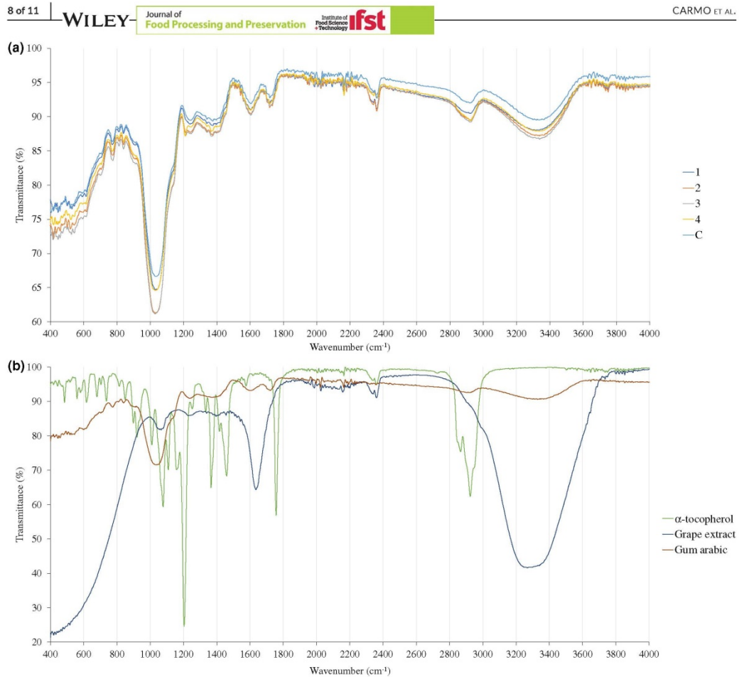
FIGURE 2 (a) FTIR spectra of the samples of each treatment and (b) the individual constituents of the microparticles (grape extract, \alpha -tocopherol, and gum arabic). C corresponds to the control treatment (no \alpha -tocopherol added), whereas 1, 2, 3, and 4 are the treatments containing 0.5, 1.0, 1.5 and 2.0% (w/w) \alpha -tocopherol, respectively
