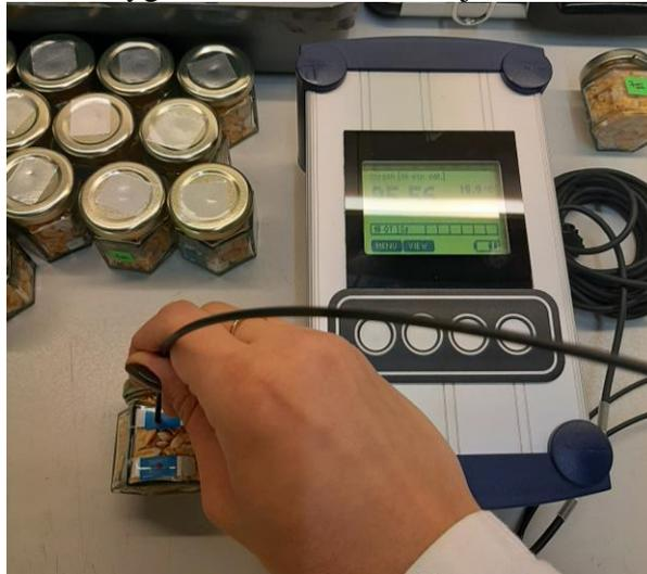
Figure 3 - Measurements of oxygen and carbon dioxide concentrations using gas analyzer Oxybaby.
