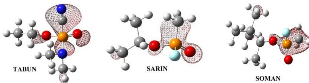
Figure 9. LUMO orbitals formation for each nerve agent ( R_P enantiomer) prior to the hydrolysis reaction to take place.
