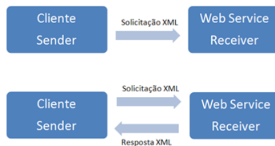
Figura 4: Modelos One-Way e Request-Response Messaging . [12]
