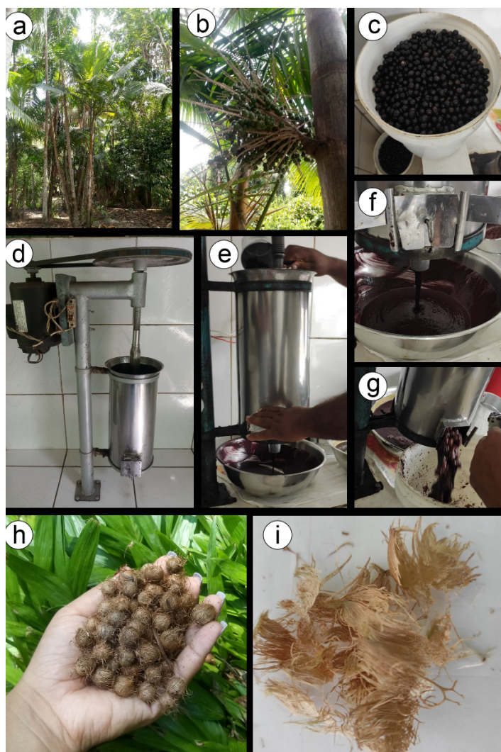
Fig. 1 Açai from the forest to urban waste: a) açai palm; b) fruit bunch; c) mature fruit; d) depulping machine; e) depulping processing; f) edible pulp; g) waste generation; h) clean waste (seeds + surface lignocellulosic fibers); and i) waste mesocarp fibers handily removed from the seeds, the studied feedstock.
