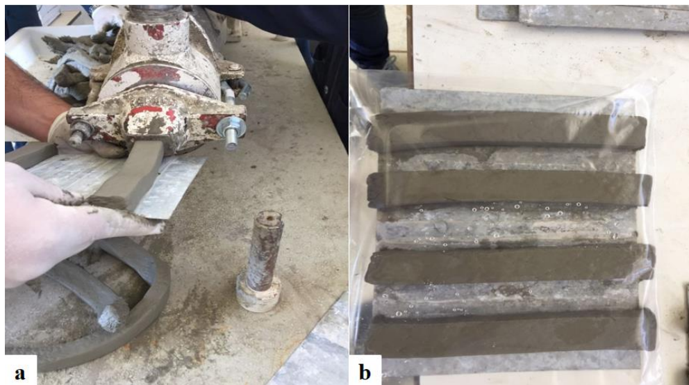
Fig. 1 Extruded fiber-cement molding process. (a) Specimen output through the extruder nozzle; (b) Specimens wrapped in a plastic bag containing water inside for the wet curing period
