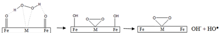
Fig.14 Route 1, less favorable to the generation of \text{HO}^\bullet radicals from the \text{H}_2\text{O}_2 decomposition on the catalyst surface.
