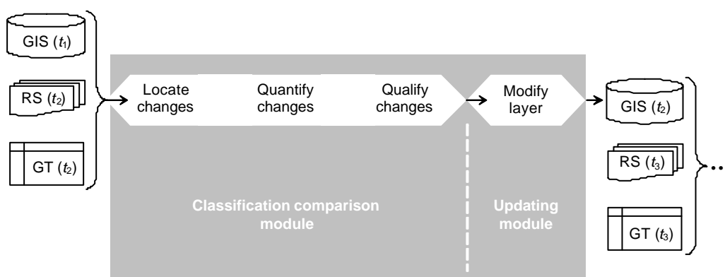
Figure 2. Flow diagram illustrating post classification comparison.
