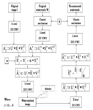
Figure 1: The diagram of the embedding and extracting process.
