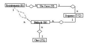
Figure 1: Requirement to UML model mapping: UML Relationships
