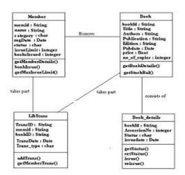
Figure 4: Class Diagram of LMS
