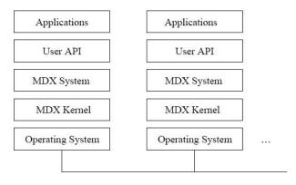
Figura 3: The basic architecture of the MDX system over a network
