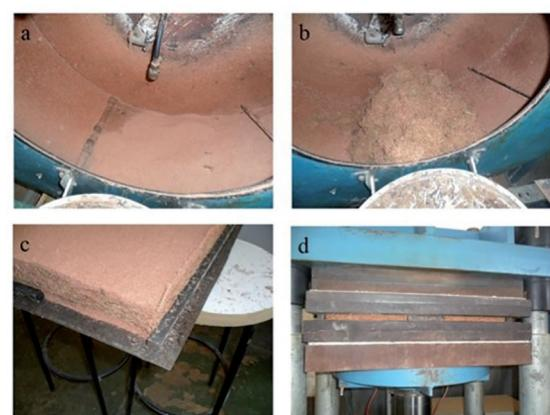
**Figure 1:** MDP production. (a) Adhesive application to smaller particles. (b) Adhesive application to bigger particles plus fibers. (c) Particle mattress after the pre-pressing. (d) Particle mattress during the hot press.
