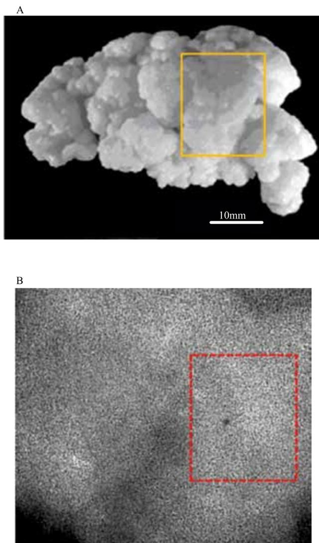
**Figure 1.** Biological activity of kefir grains by laser biospeckle technique: A, kefir grains; B, image formed by laser biospeckle (captured by a CCD camera of 640 × 486 pixels (Systems Ltd, Chennai, India), with a shutter speed of 1/60 s at rate of 0.08 s).
