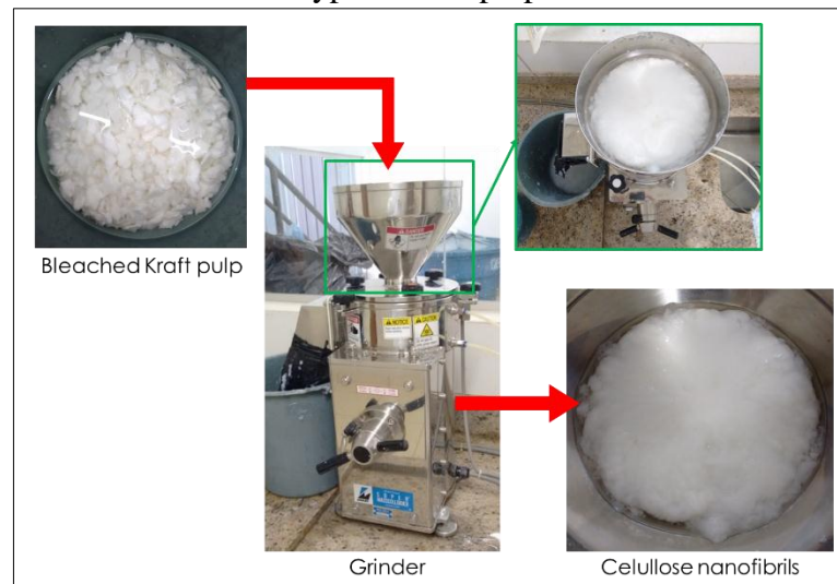
Figure 1 - Bleached eucalyptus Kraft pulp mechanical defibrillation.
