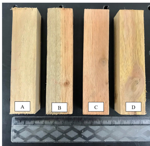
Figure 2. Samples in different classes of knots. A: clear wood; B: class 1; C: class 2; D: class 3.
