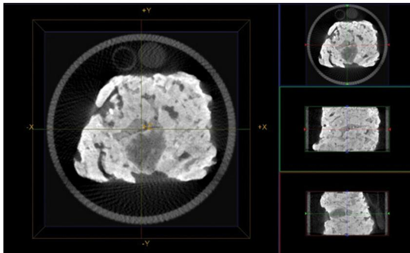
**Figure 3.** Cross-section of an ironstone fragment ( $47 \times 38$  mm, in the XY axis) showing “vermicular” porosity, large irregular partially infilled pores, and dense masses (bright areas) on the outer rims or isolated grains. The large image shows the combination of the X, Y, and Z (Z orthogonal to XY) axes. The smaller images show, from top to bottom, the XY, XZ, and ZY planes.
