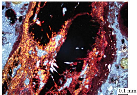
**Figure 1.** Thin section of the A horizon of the Petroferric Acrudox, showing the opaque cores of a dismantling ironstone, surrounded by a partially deferrified matrix (bright red and orange masses). The fragment appears to disintegrate, creating a friable outer rim of brown colors, which seems to give rise to the microgranular peds within the packing voids (blue colors). Image taken between partly crossed polarizers.
