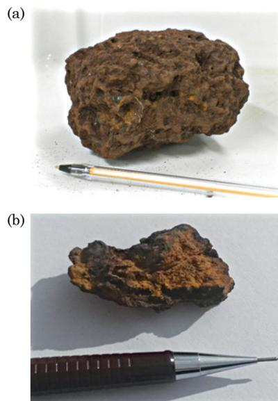
**Figure 2.** (a) Natural fragment of ironstone used for bulk and particle density determination (note root remains on the surface); (b) ironstone fragment showing a black color due to predominance of macrocrystalline Fe oxides, and yellowish masses suggesting oxide hydration and disintegration.
