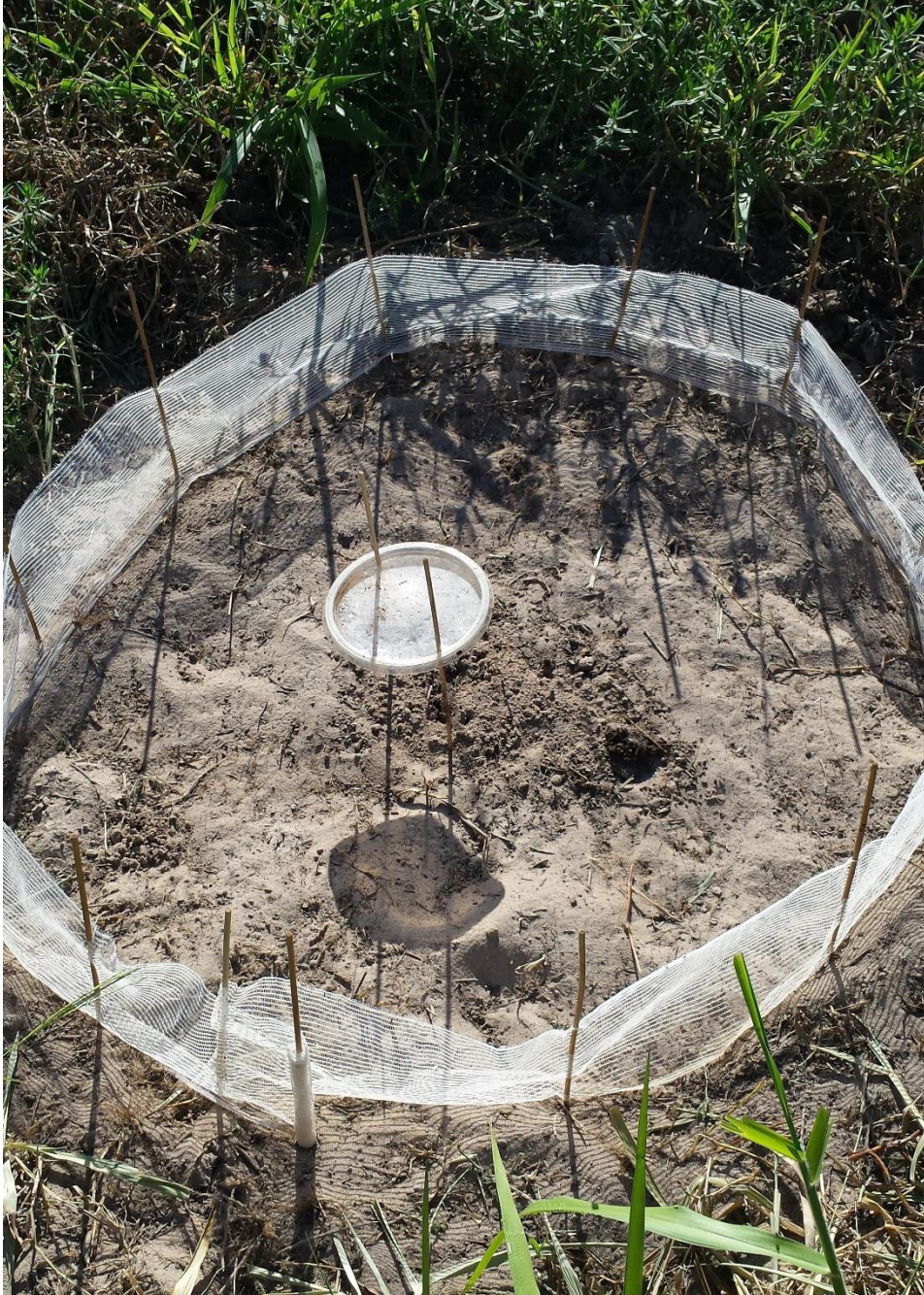
Fig. S1 Experimental arena used for measuring the dung beetles ecological functions: dung removal and soil bioturbation (see main text for description).
