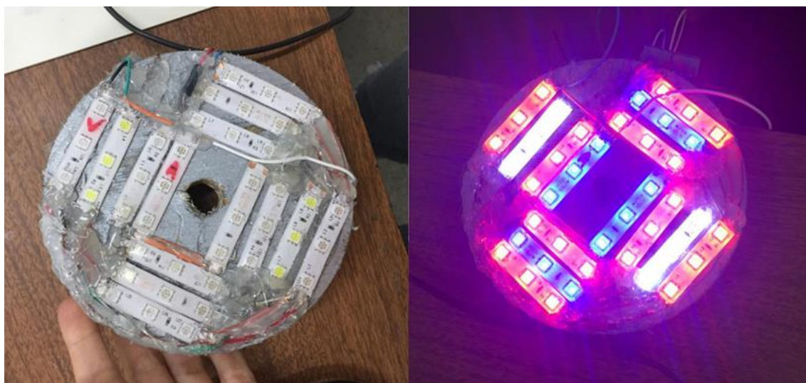
Figura 10 – Placa de luz mostrando as fitas de LED instaladas
