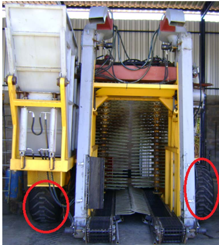
Figure 11. Coffee harvester machine with misaligned rear wheels in operation.
