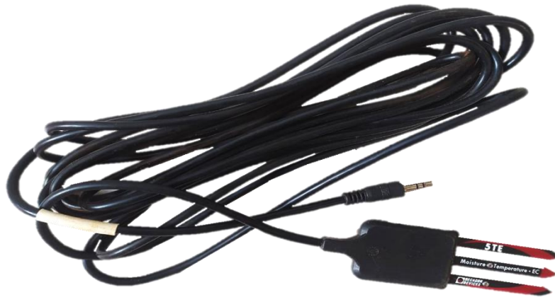
Figura 4 – Sensor 5TE da Decagon®, Volumetric Water Content (VWC), Temperature, and Electrical Conductivity (EC) sensor from METER Group.
