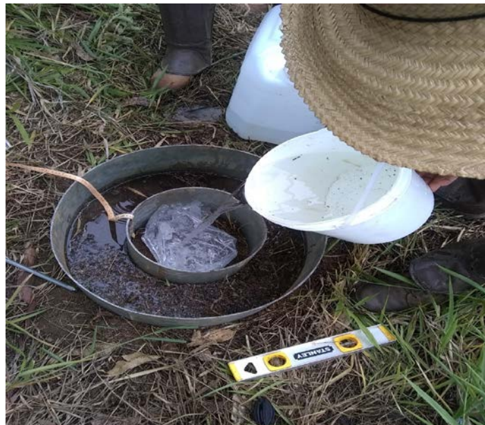
Figure 5 – Double ring infiltrometer used in the soil water infiltration rate test.
