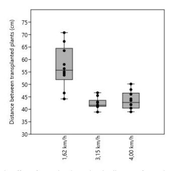
Figure 2. Boxplot for the effect of operational speed at the distance of transplanted seedlings
