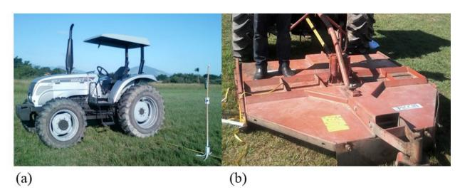
Figure 1. Agricultural tractor measured for noise levels: a) without activation of a rotary cutter; b) with activation of a rotary cutter.
