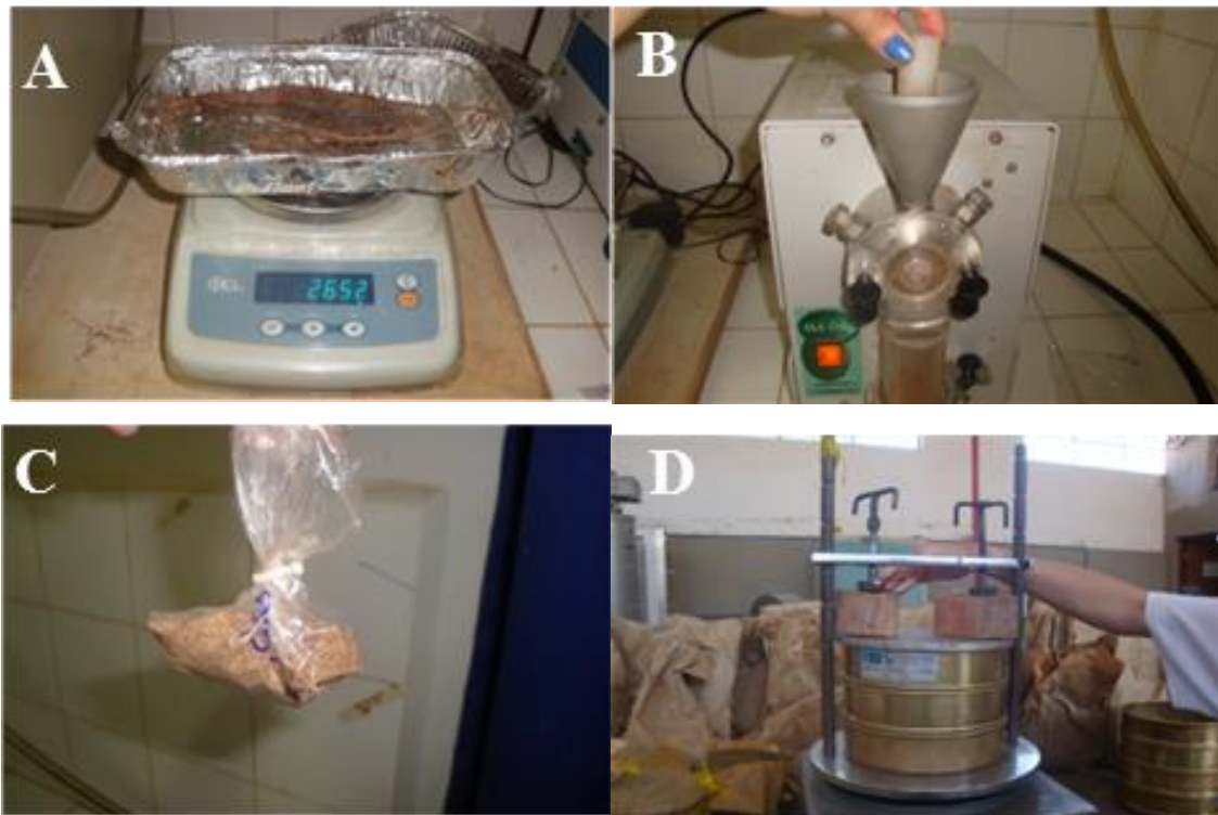
Figure 4. (A) Weighing the samples in a scale; (B) Grinding the samples in Wiley mill; (C) Sampling after grinding; (D) Classification of samples in 200 and 270 mesh sieves.
