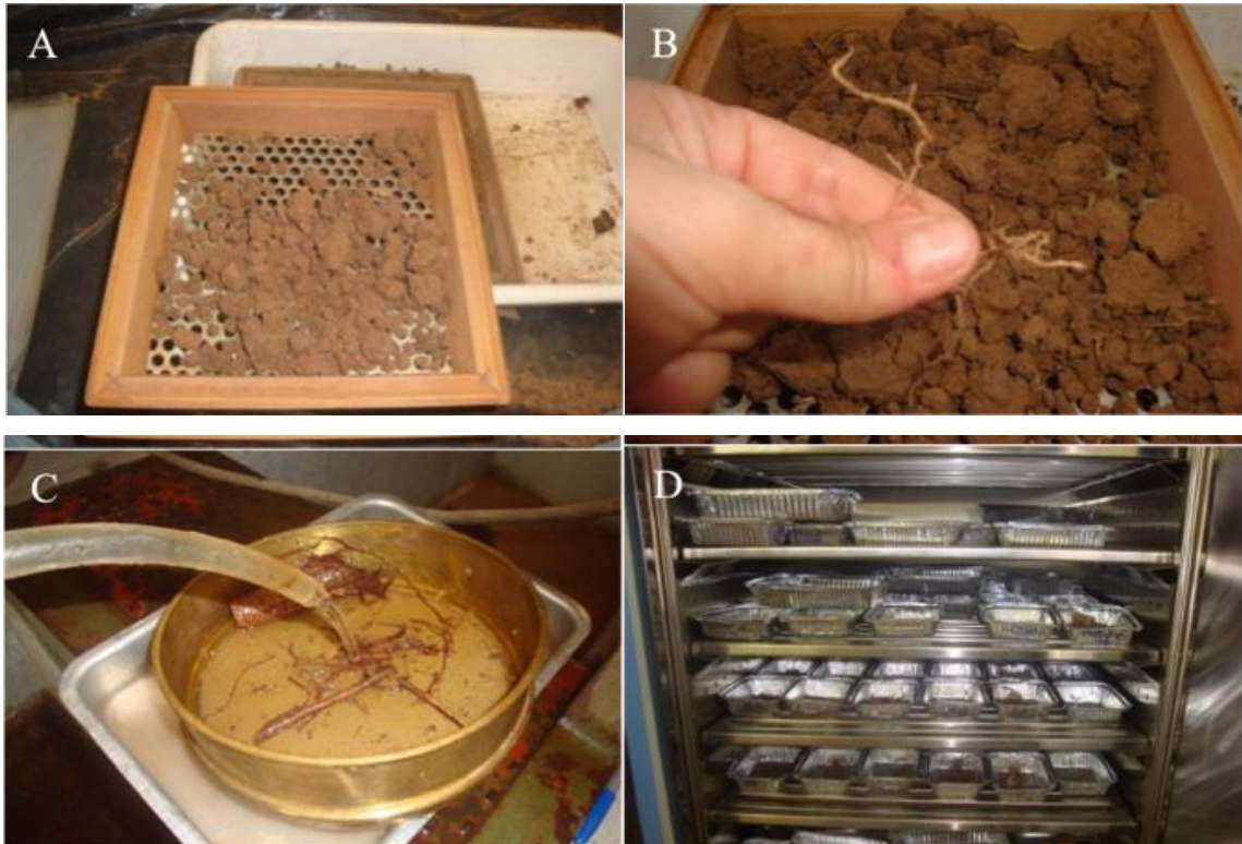
Figure 3. (A) Root separation; (B) Root of Anadenanthera sp.; (C) Root wash; (D) Samples packed in the oven.
