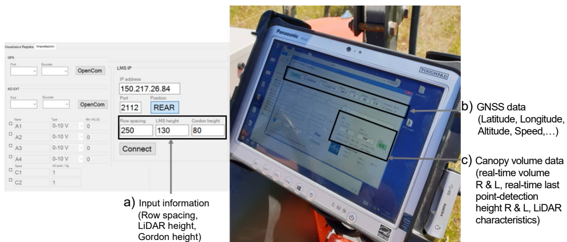
Figure 3. Software interface for computing, in real-time, canopy volumes. On the left, the interface window, that allows to set parameters about LiDAR position and vineyard characteristics was shown. On the right, there is the working window, where canopy volumes (right and left side) and canopy heights were shown in real-time.
