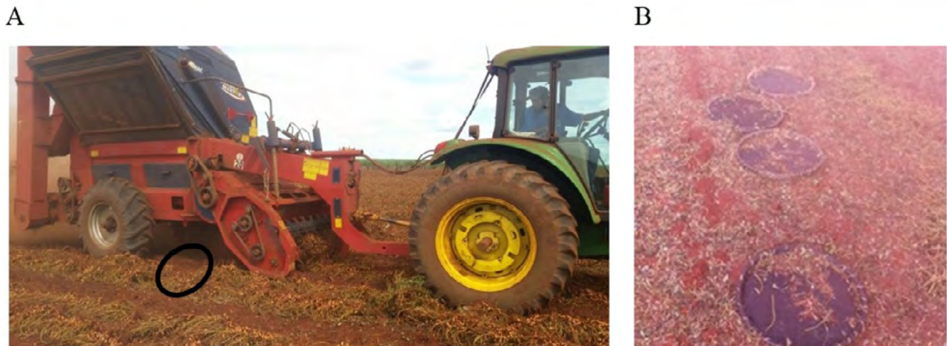
Figure 2. Methodology example to evaluate losses in peanut combining. The black circle represents frames being thrown between the platform and the peanut combine wheels axis, in movement (A). Frames arrangement after passing of peanut combine (B).
