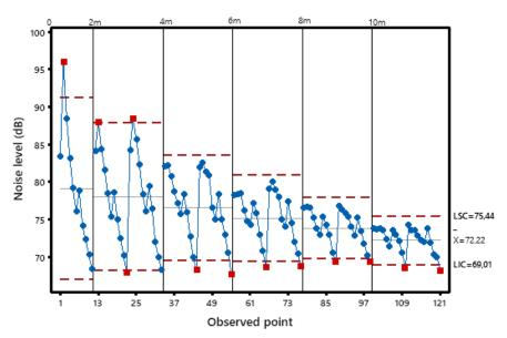
Figure 6. Control chart for the noise levels of the backhoe
