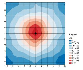
**Figure 3.** Spatial distribution map of the noise produced by the backhoe
