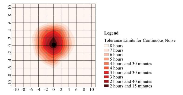
Figure 4. Spatial distribution map of the period of exposition to the noise produced by the assessed tractor
