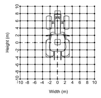
**Figure 1.** Sample grid of the levels of noise produced by the backhoe. The dark dots are the sample points
