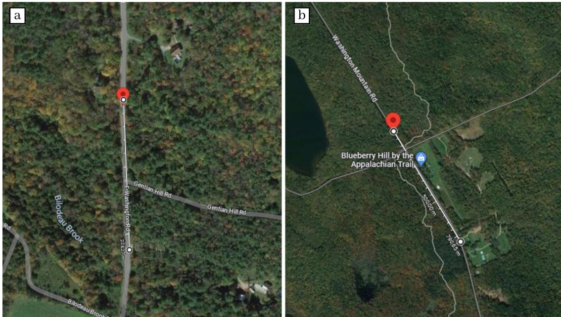
Fig 19. Distance to the nearest curve. Example: a) a curve in the segment of 500m than the value was 0; b) a curve at 790m distant from the centroid.
