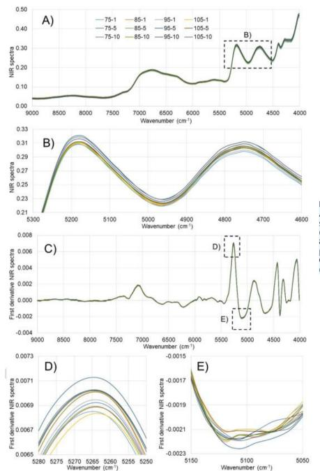
**Figure 2.** Mean raw (untreated, A) and first derivative (C) NIR spectra for each nanofibril content (1, 5 and 10%) and grammage (75, 85, 95 and 105 g m<sup>-2</sup>) of Kraft paper handsheets reinforced with CNF and detailed spectra ranges (B, D and D).
