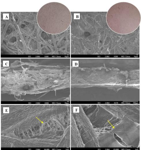
**Figure 1.** FEG-SEM micrographs of papers reinforced with cellulose nanofibrils showing paper surfaces rough (A) and smooth (B) with respective samples, paper thickness (C, D), formation of nanofilm within the paper (E, F). Arrows pointing to zones of nanofilm formation.
