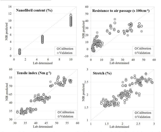
Figure 5. Lab determined versus NIR Spectroscopy predicted values to estimate physical and mechanical properties of paper reinforced with CNF.
