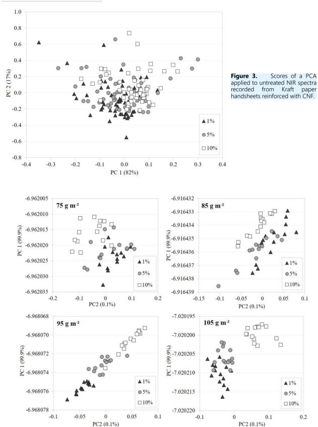
Scores of PCAs applied to NIR spectra after Multiplicative Scatter Correction recorded from Kraft paper Figure 4. handsheets reinforced with CNF with nominal grammage of 75, 85, 95 and 105 g. m<sup>-2</sup>.
