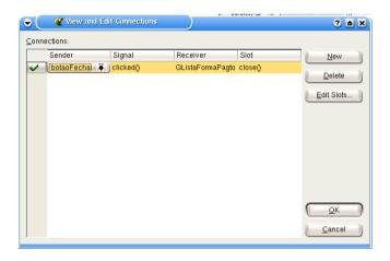
Figura 6-14. Designer - conectando signal e slot
