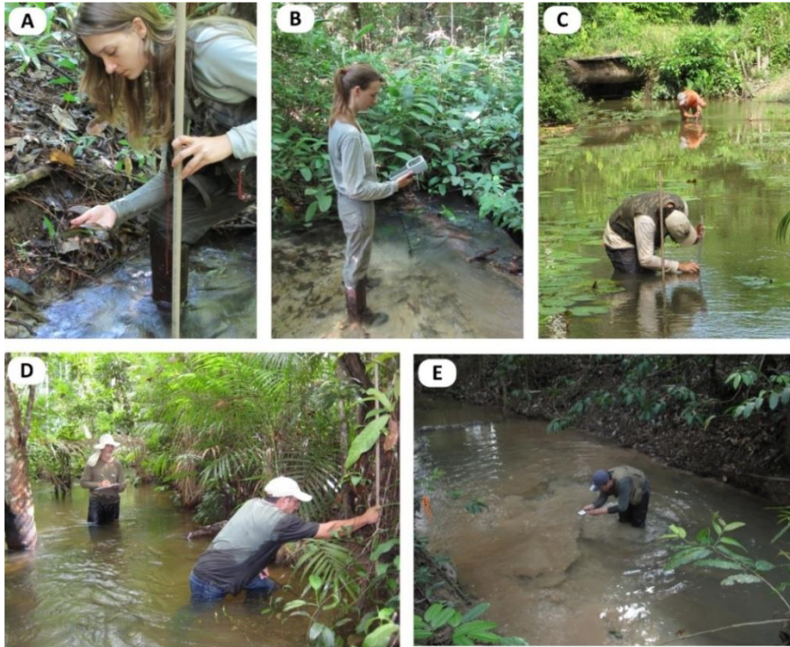
Figure 1.7 Measuring instream habitat characteristics in stream sites: substrate type (A), water properties (B), channel slope (C), depth (D), and canopy density (E). All pictures by RAS Aquatic Team.
