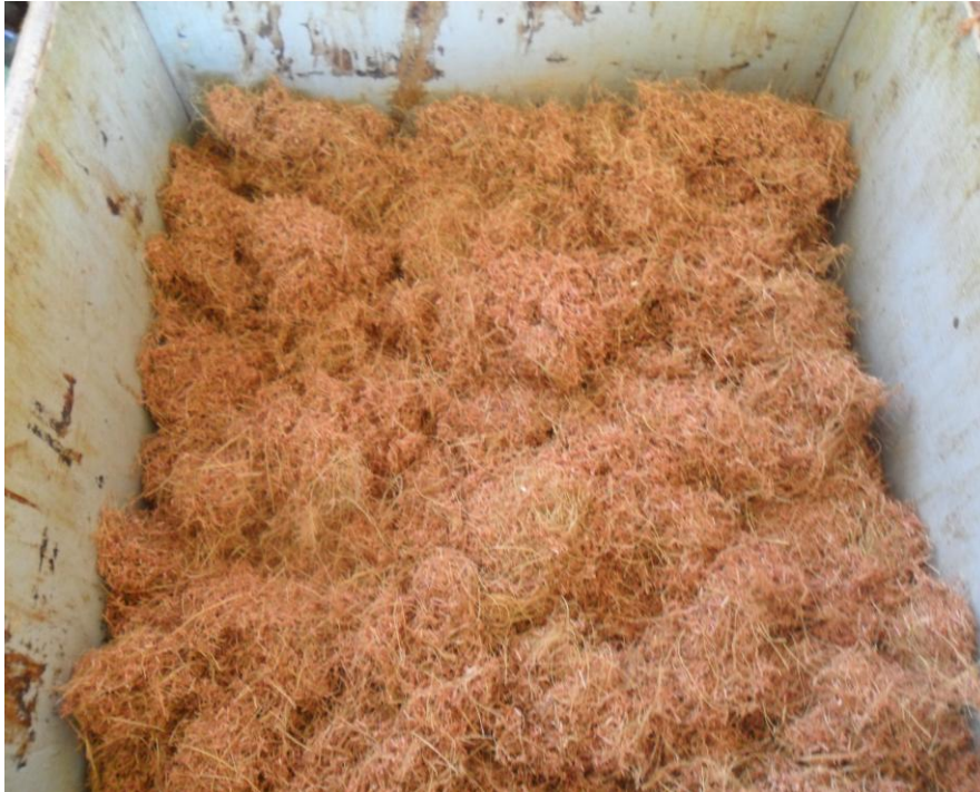
Figure 5 - Clumps formation during the adhesive dispersion and the mattress formation
