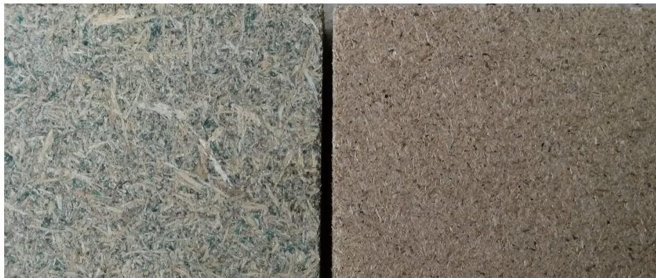
Figure 7 Commercial SCB particleboards from China with longer particles (in the right) and SCB particleboards made in the present work (in the left)
