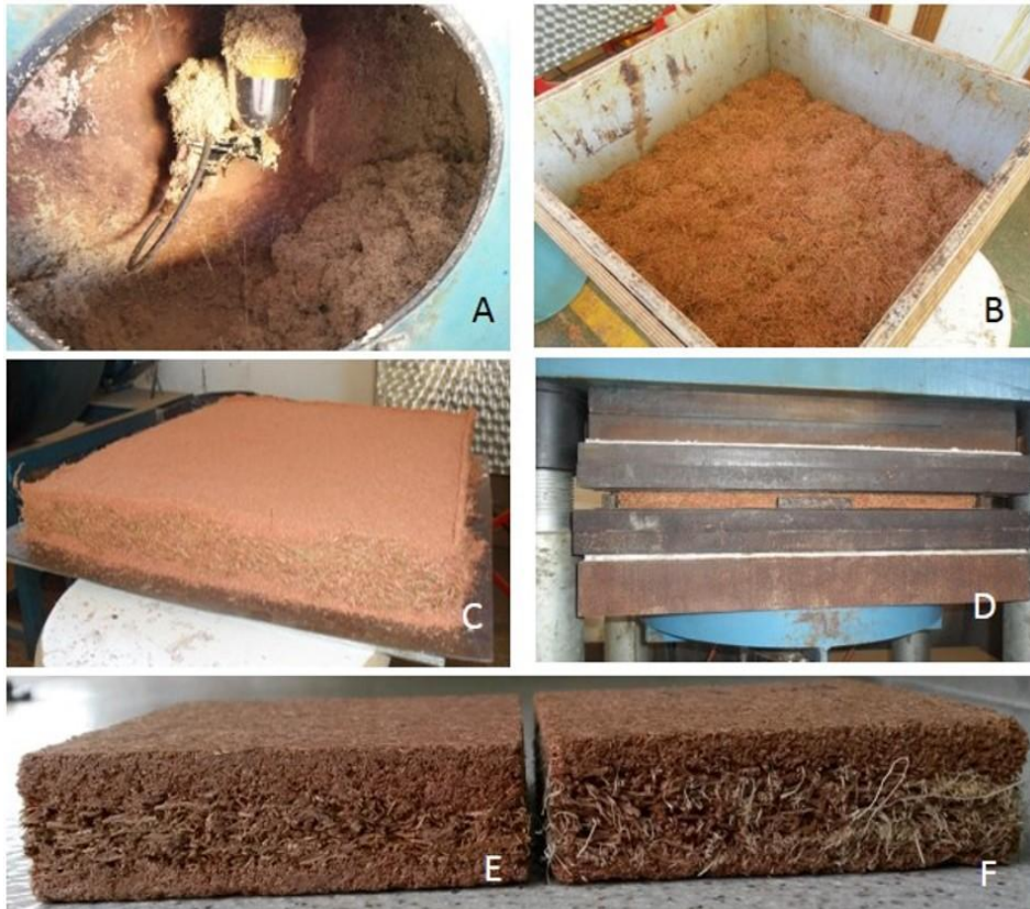
Figure A 1 F Particleboard production. A – Adhesive application. B – Particle mattress formation. C - Particle mattress after pre pressing. D – Hot pressing. E – Particleboard with 20% of coir. F – Particleboard with 20% of sisal.
