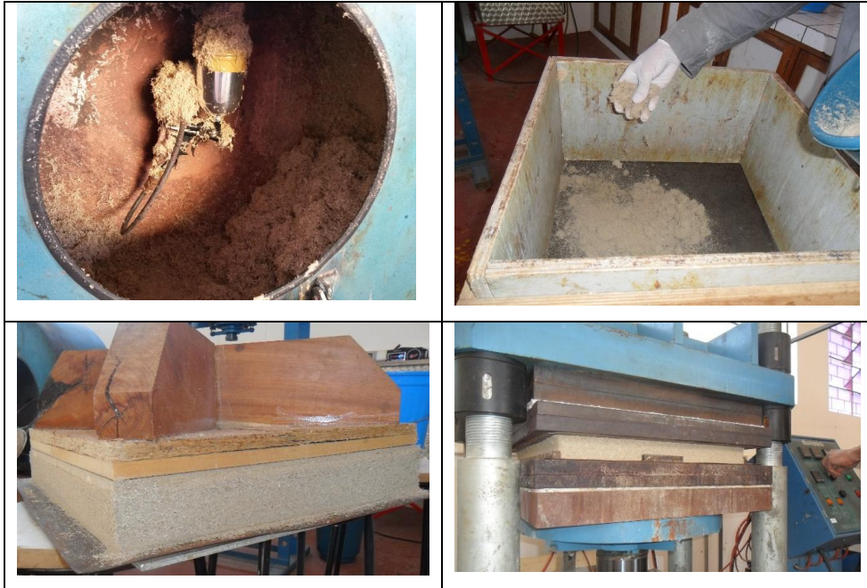
Figure 2 Particleboard production. Adhesive dispersion, particle mattress formation, mattress after pre pressing and hot pressing.
