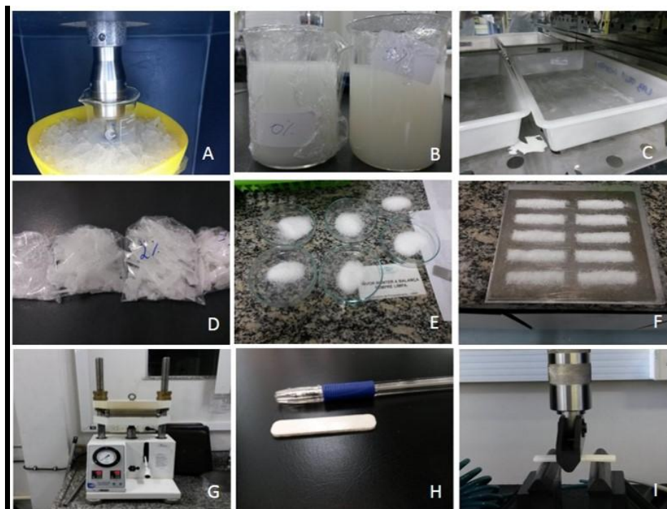
Figure B 1 Production of UF composites. A – NCC dispersion. B – Adhesive with 0% of NCC and with 5% of NCC. C – Adhesive being dried. D – Adhesive dried. E – Adhesive milled. F – UF pellets in the iron mold. G – Hot pressing. H – UF composite. I Bending test.
