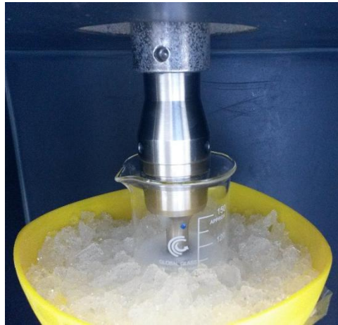
Figure 1 Beaker immerse in ice for NCC dispersion using a Branson digital sonifier.
