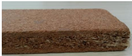
Medium density particleboard – MDP in three layers with sisal inclusion in the core
