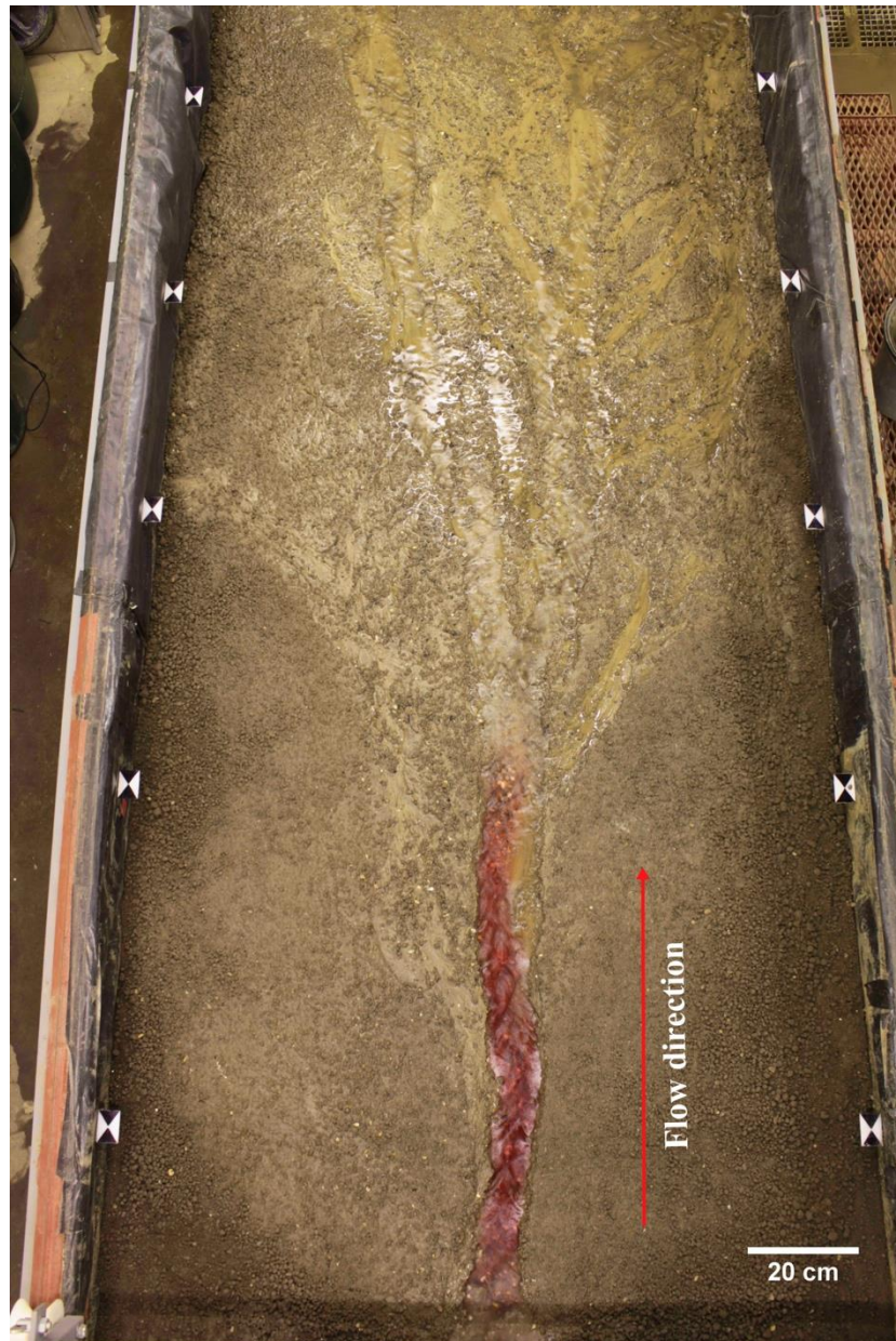
Fig. 4. Dye-pigmented water flow used as tracer for flow velocity calculations. At the sides of the experimental slope, photogrammetric control points for georeferencing the cloud of points can be seen.
